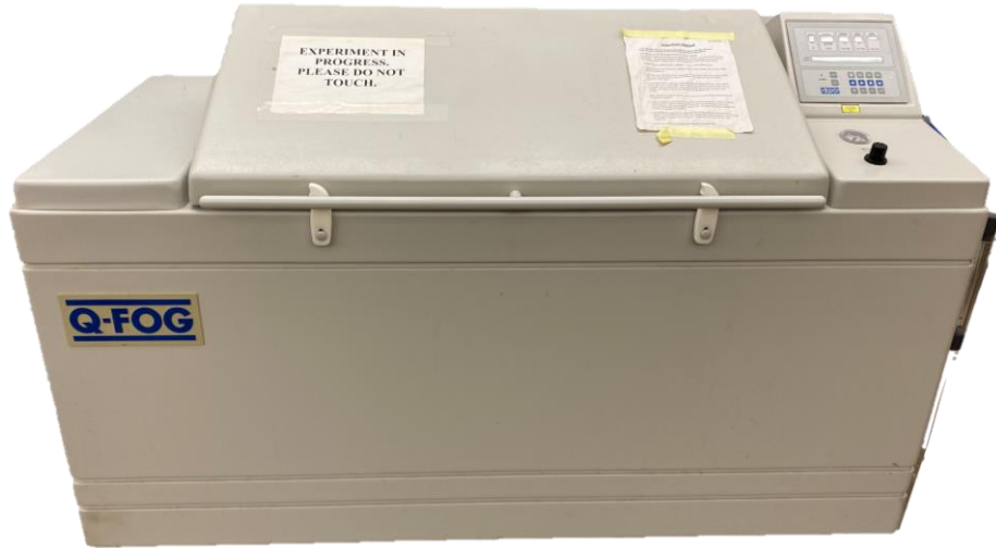
Accelerated Corrosion Chamber Q-Fog CCT-600
